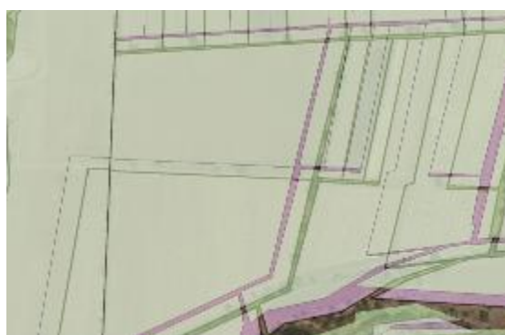
Figure 1: Shift effect observed by the different geodetic reference systems in shape files.
