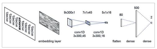
Figure 7 - The topology of the Conv1D CNN used within the proposed False Positive Reduction framework (a)
