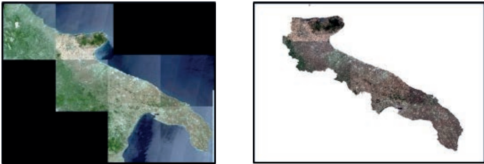
Figure 2.1 - On the left, mosaic of Apulia Sentinel-2 satellite images. On the right, the same mosaic clipped by the Apulia boundaries
