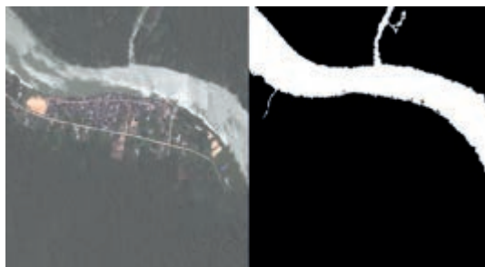
Figure 3.5 - Example of river segmentation by a U-Net model
