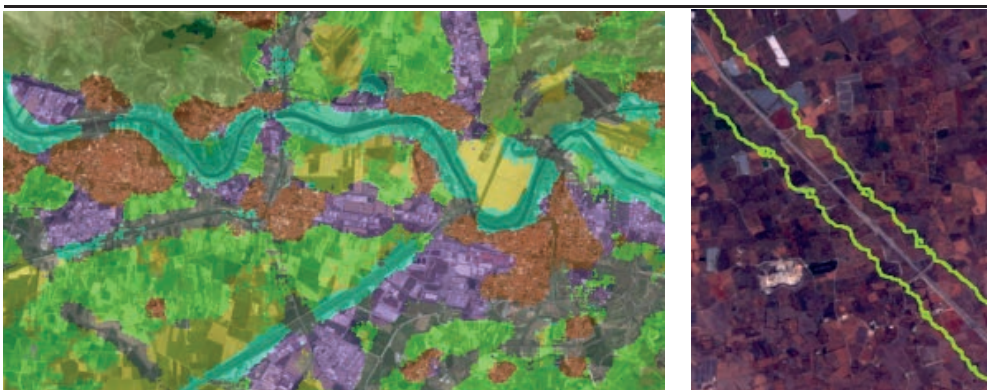
Figure 3.2 - Visual illustration of the overestimation issue affecting our system with respect to LC classes ‘River’ (left panel: bends of river Arno, cropped from the north-east quadrant of the ‘Pisa image’) and ‘Highway’ (right panel: a fragment of a highway cropped from the south-east quadrant of the ‘Lecce image’)
